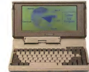
TI200HB: 10.8 lbs, 9.54MHz 80C86, 20MB hard disk, 1MB RAM, includes 384KB LIM-EMS. Removable/rechargeable battery pack.
